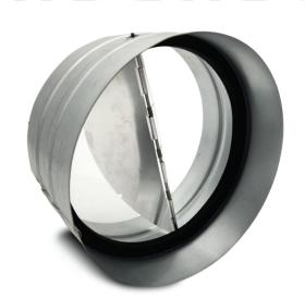
Alpine Ventilation has a range of inline butterfly dampers to prevent backdrafts in ducting. They are constructed with galvanised steel, with 2 spring loaded aluminium dampers and a foam ring for quiet operation. The damper goes inside ducting and secures with worm clamps and/or duct tape.
