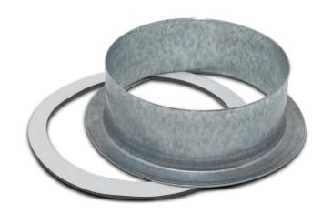
Alpine Ventilation has a range of round flange adapters in 3 sizes. These are used for an application where there is no neck to connect to, using the double sided adhesive foam ring to attach adapter to surface. The 100mm size is generally used for clothes dryers and the 125mm and 150mm sizes generally used for rangehoods.
