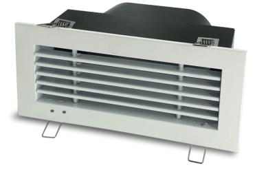
Alpine Ventilation has developed a stylish aluminium bar grille for bathrooms and laundries. Used with an inline axial fan, it is an ideal alternative to exhaust fans with a built in grille. A 150mm adapter connects directly to ducting. Using a grille with separate inline fan reduces noise when compared to a regular exhaust fan with grille.
